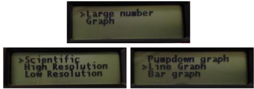
Display modes are selected from the display menu Display, and numeric formats are selected from the Setting option "Display". The SEL button enters and traverses the Settings menu.
